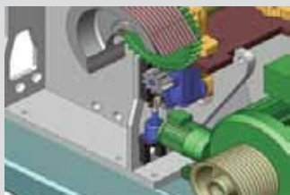
Slow rotation by gearmotor
