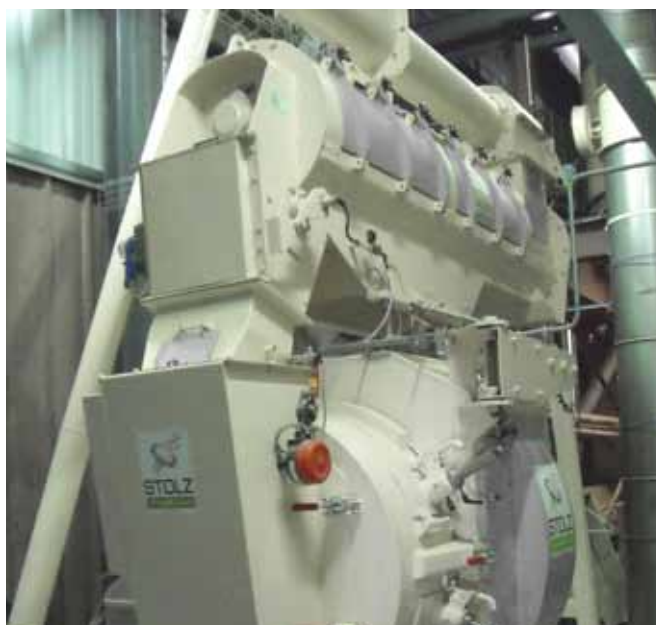
Long residence time horizontal conditioner on pellet mill
