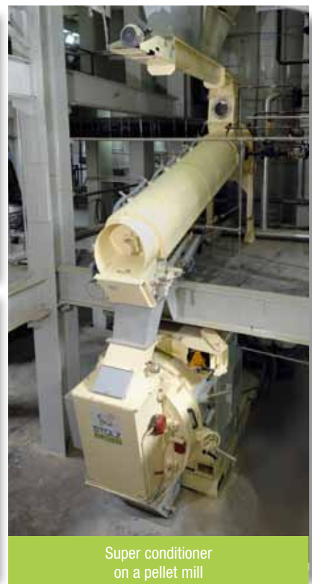
Super conditioner with steam injection
