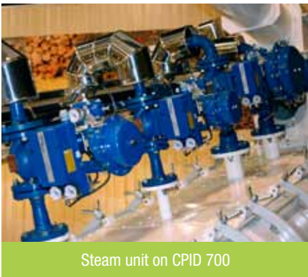
Super conditioner with steam injection
