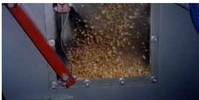
Adjustable flap for air/product segregation
