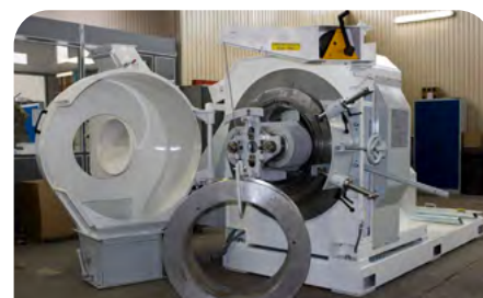
Built-in winch for die handling
