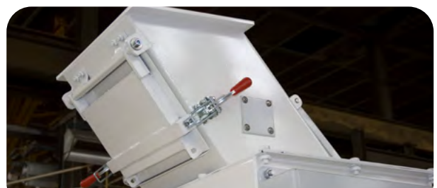
Magnet plate on feed duct
