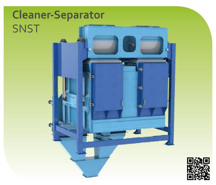
The operating principle of the SNST is simple and effective. The seed or other product comes by a dispatching device over the whole width of the sieve. The efficiency of screening is increased significantly by weighted rubber balls to ensure the cleaning of the whole working surface area without wearing screens.
