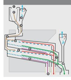
The product introduced into inlet **1** drops into a distribution trough **2** balanced with counterweight then slides in layer into a suction duct **3** equipped with four diverters **3**. The sifting module is subjected to a circular movement. It includes a spreading chamber followed by two sifting levels. The product goes through a spreading device with 2 levels **3** feeding the coarse sieves **3** tilted at 9°.
